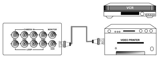
Connect VCR or VIDEO Printer to VCR out on the rear panel of Built in DVR.
